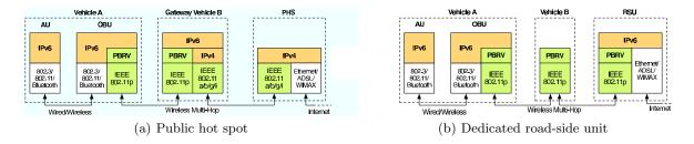
Fig. 2. Resulting protocol architecture
