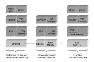
Fig. 2. Protocol architecture for communication-based intersection safety.
