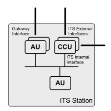
Fig. 3: ITS Station components
