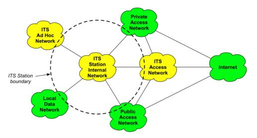
Fig. 4: ITS network architecture
