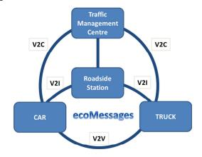
Figure 1 eCoMessages in the System Architecture (v: vehicle, i: infrastructure, c: center station)
