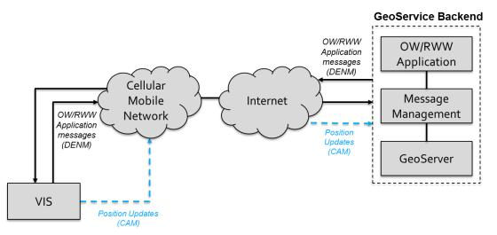
Figure 2 – Information flow between VIS and GeoService Backend
