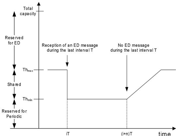
Figure 2: DRCV Fast Drop scheme
