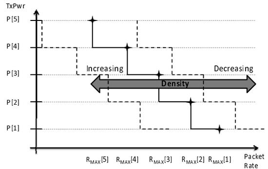
Fig. 1. Rate-power relation in power+rate control.
