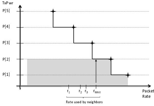
Fig. 2. Beacon rate selection in power+rate control.
