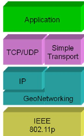
Figure 2: Protocol architecture of distributed vehicular communication.
