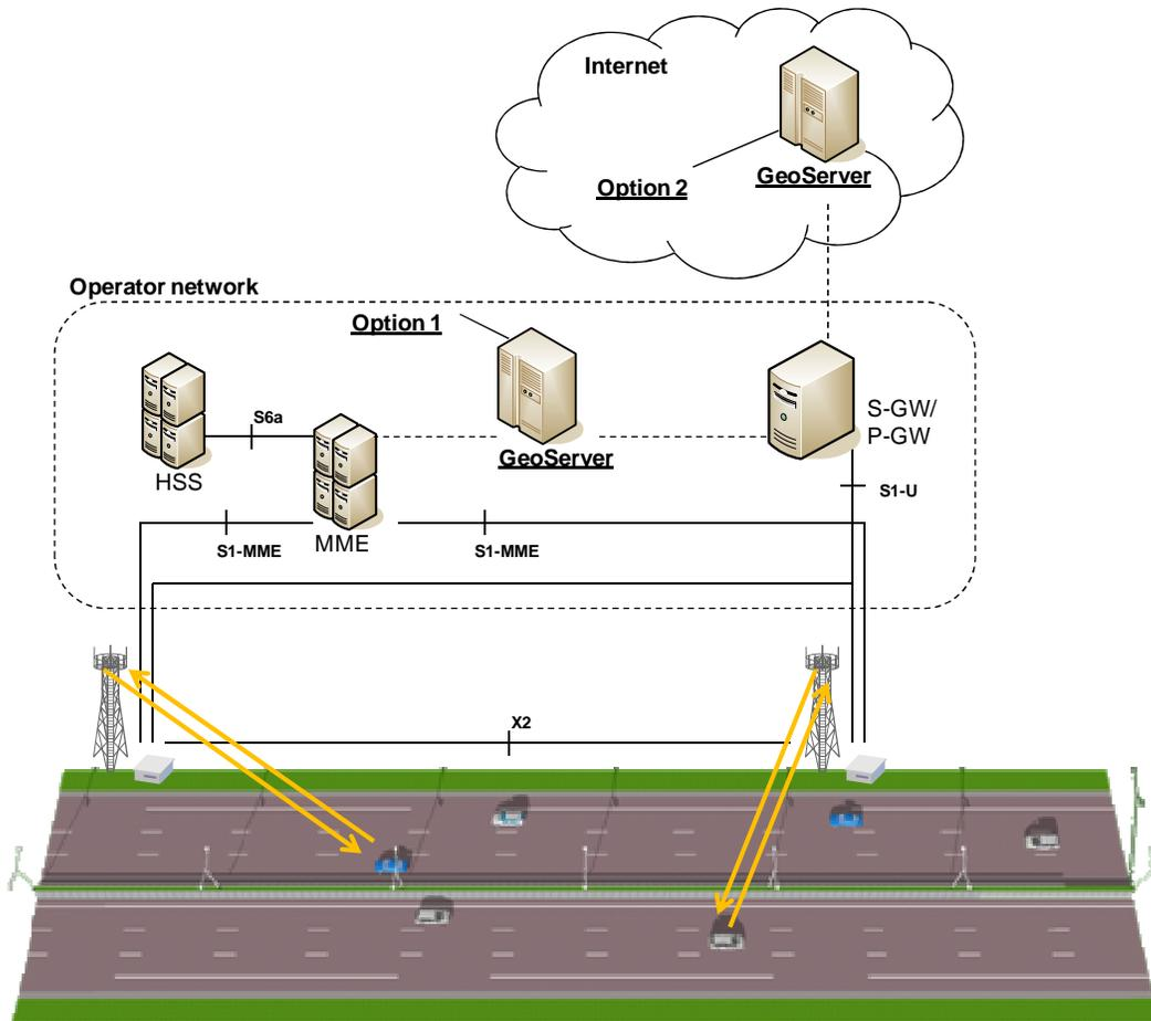
Figure 5: System architecture options for centralized vehicular communication.
