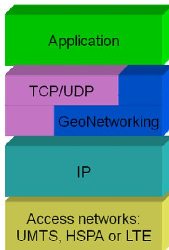
Figure 4: Protocol architecture of centralized vehicular communication.
