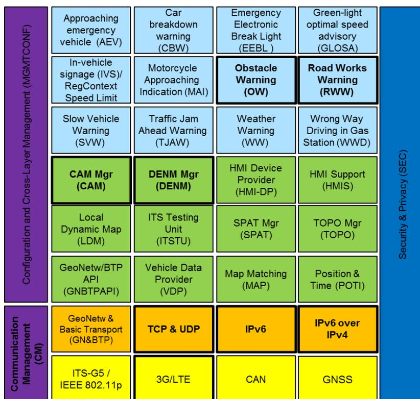
**Figure 4:** VIS Implementation design in DRIVE C2X
