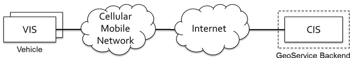
**Figure 1 - System architecture for RWW/OW applications over cellular mobile networks**
