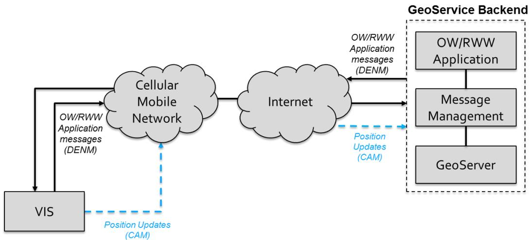
**Figure 2 – Information flow between VIS and GeoService Backend**
