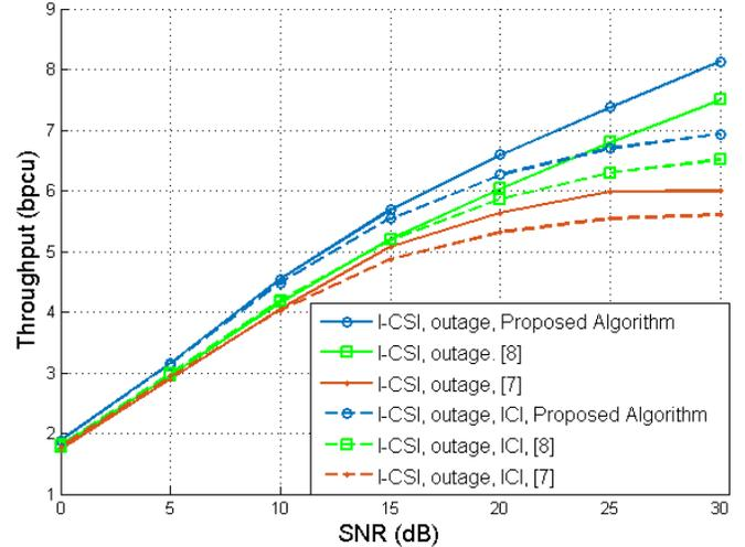
Fig. 3. Throughput in *bpcu* against SNR considering outage with/without inter-cluster interference for various algorithms
