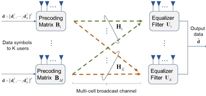
Fig. 2. Model of a cooperative multi-cell MIMO system
