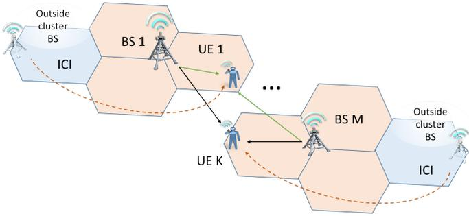
Fig. 1. A cellular system structure for cooperative multi-cell transmission in the downlink
