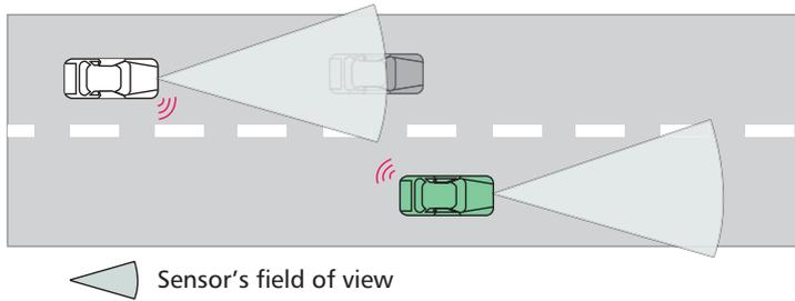
**Figure 3.** Exchange of detected objects for cooperative sensing.
