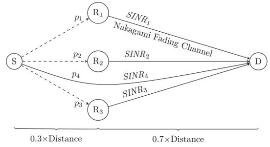
Fig. 3. Simulation scenario for the evaluation of enhanced CBGF. The source  $S$  sends packets to the destination  $D$ , which decodes the packet with the assistance of the relays  $R_i$ . The packets received by  $R_i$  can have errors (indicated by the bit error rates  $p_i$  and the dashed lines); nevertheless they are forwarded. The direct link is modeled with  $p_4 = 0$  and  $SINR_4$ .
