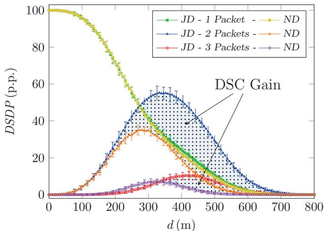
Fig. 8. Division of successfully decoded packets,  $DSDP$  for joint decoding (JD) and normal decoding (ND) with three relays. As an example, at distance  $d = 400$  m the overall  $PSR$  is about 85% from which 25 percentage points (p.p.) were successfully decoded with a single packet copy ( $DSDP = 25$  p.p.), 50 p.p. with two copies and 10 p.p. with three copies at the destination.
