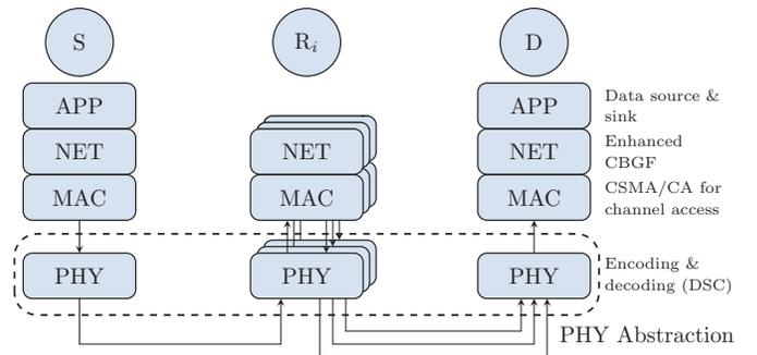
Fig. 4. Simplified protocol stack used for performance evaluation.
