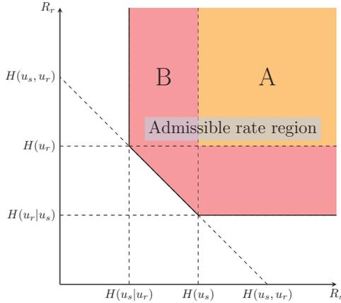
Fig. 1. Admissible rate region for successful recovery of two packets from two sources at the destination. Region A is the rate when the packets are uncorrelated and region B is the extension enabled by the Slepian-Wolf theorem.
