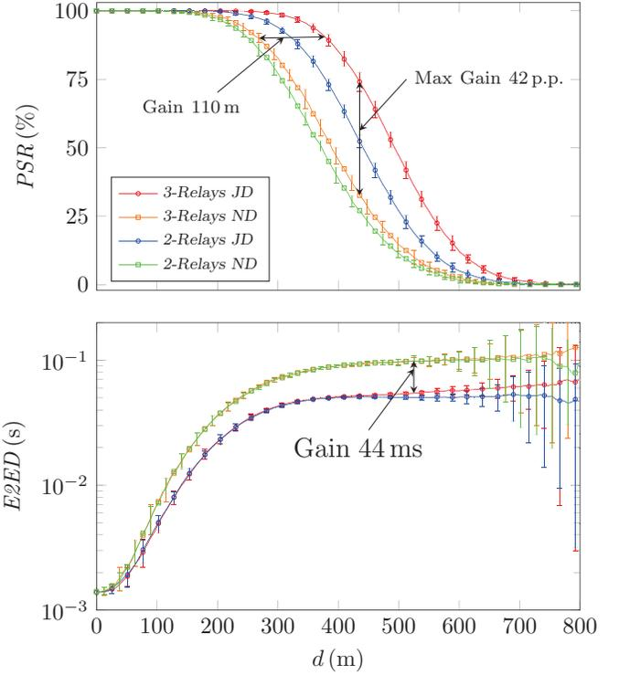
Fig. 6. Packet success ratio  $PSR$  (top) and end-to-end delay  $E2ED$  (bottom) over distance ( $d$ ) for two and three relays. Enhanced CBGF (with joint decoding – JD) and baseline CBGF (with normal decoding – NC) is exhibited.
