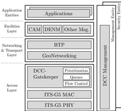
Fig. 1. DCC-gatekeeper at the access layer of the C-ITS protocol stack.
