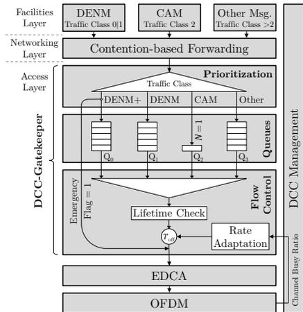
Fig. 2. Queuing system of the DCC-gatekeeper in the context of the C-ITS protocol stack.
